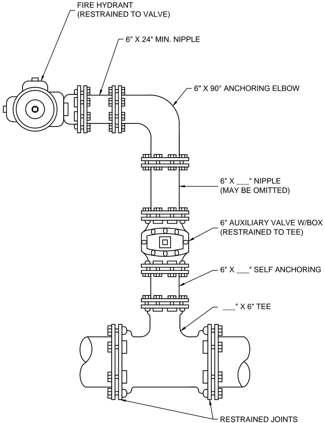
FIRE HYDRANT ASSEMBLY TYPE III MODIFIED
