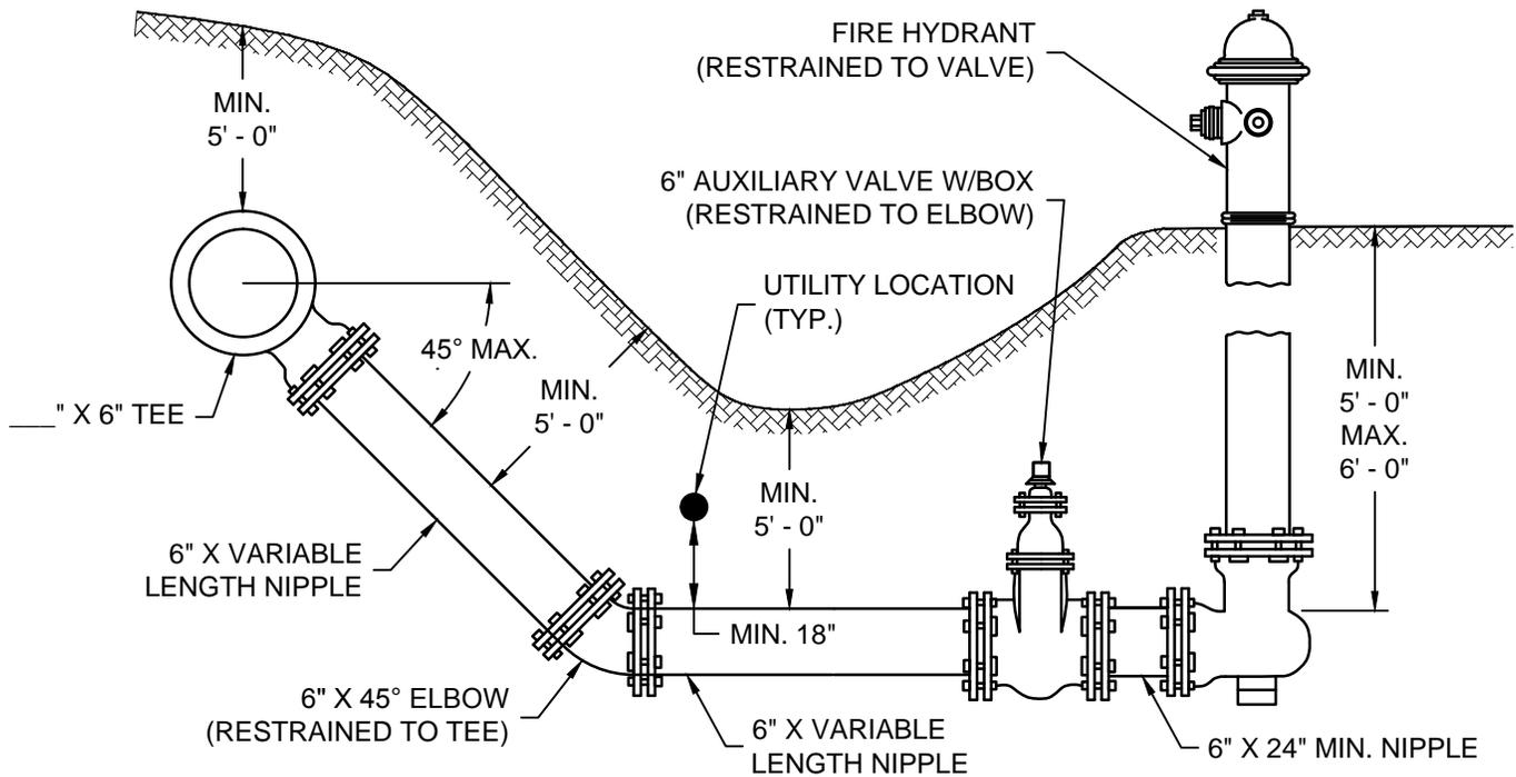
FIRE HYDRANT ASSEMBLY TYPE IV MODIFIED
