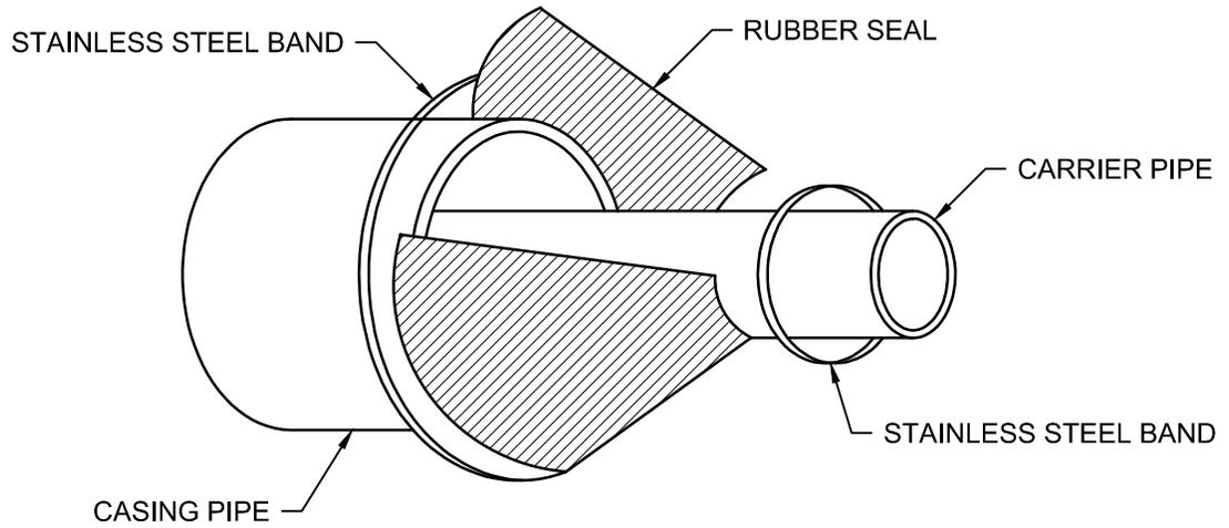
RUBBER END SEAL (3" DIAMETER AND SMALLER CARRIER PIPE)
