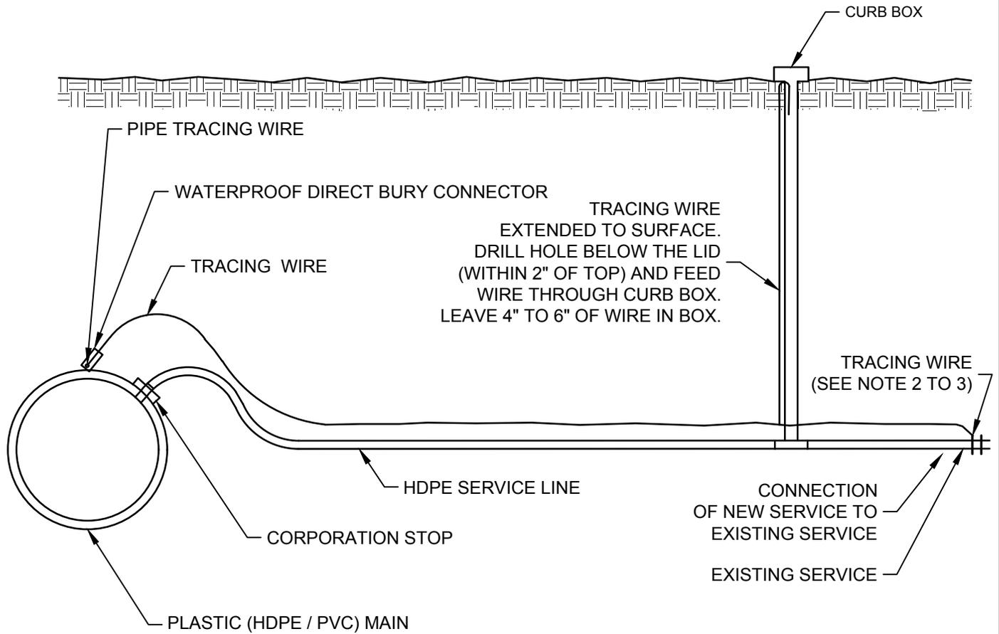
SMALL SERVICE - TRACING WIRE CONNECTION
