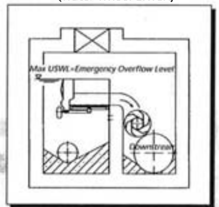
Vertical arrangement with auxiliary sill and screened material storage chamber
