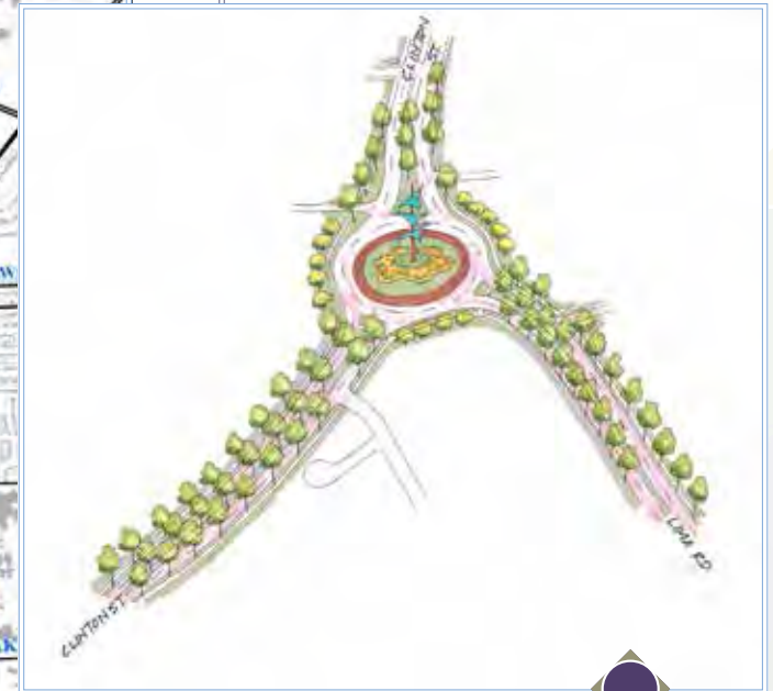
The area where Lima Road and Clinton Street intersect is awkward and can be confusing for motorists. A better solution might be to incorporate a roundabout as illustrated below.
