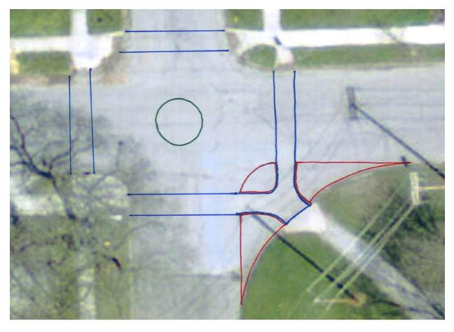
Conceptual designs do not need to be complicated or detailed. The example above shows that a few simple lines can convey a basic plan.
